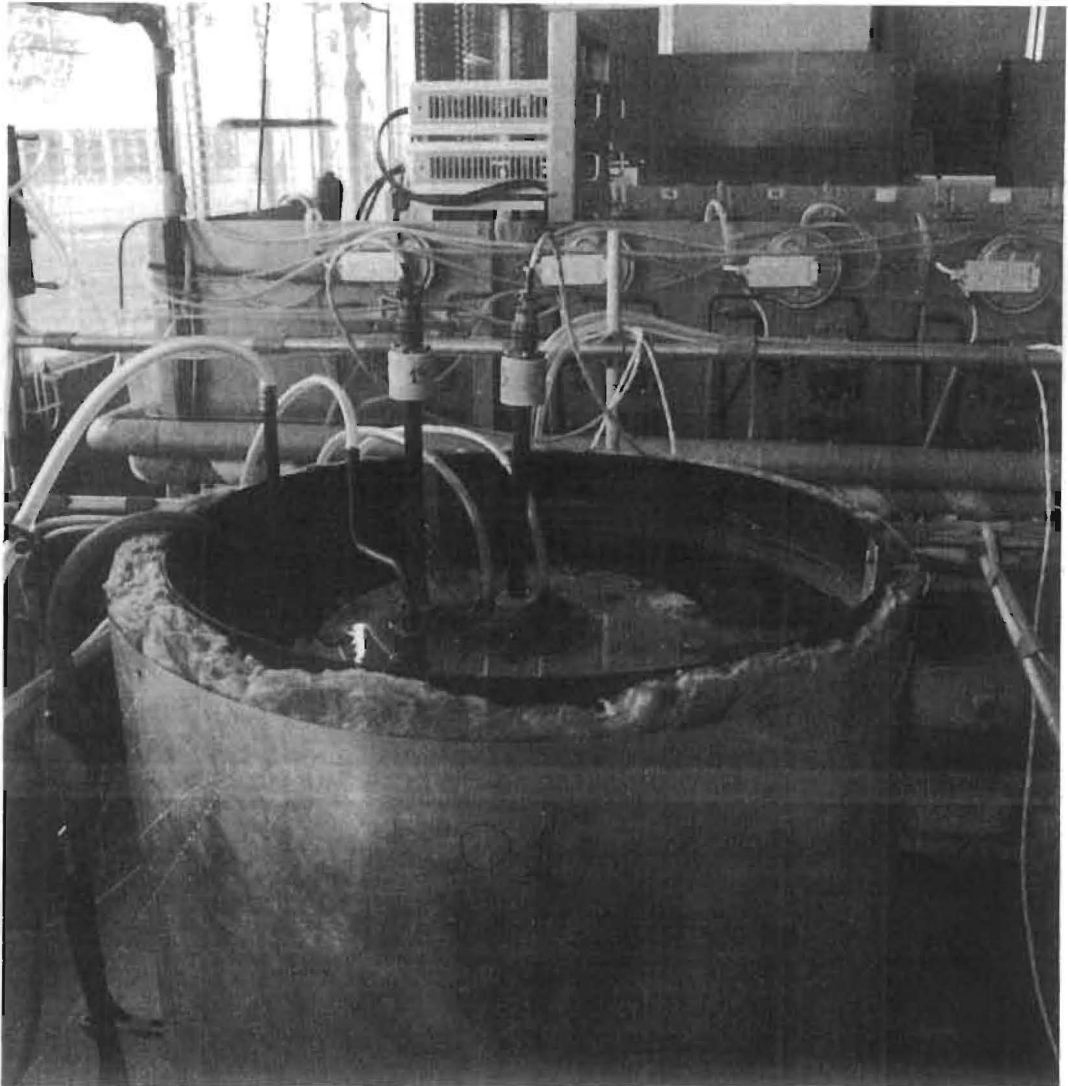
Fig.4. Adiabatic apparatus for simulation of storage conditions inside a large grain bulk.
