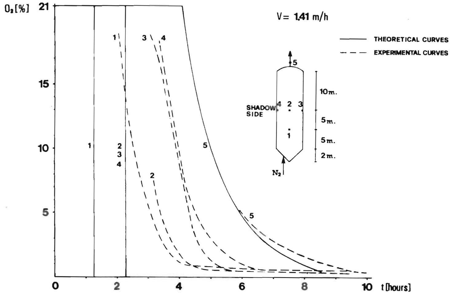
Fig.1. Comparison between theoretical and experimental results of a purging test in a SRM plant fiberglass bin at gas velocity of 1.41 m/h.
