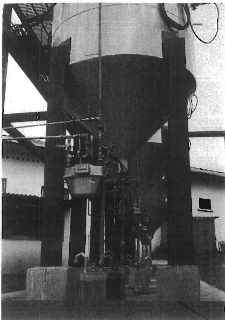
Fig.4. Pilot-scale metal storage bins with automatic interstitial nitrogen pressure maintenance device, gas meters and pressure releaf valves.
