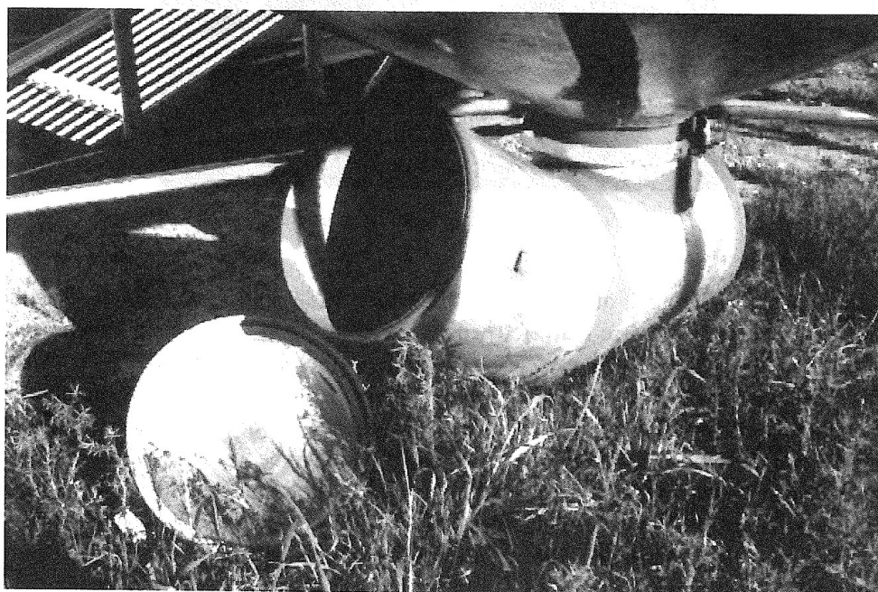
Fig. 8. Sealed rotating boot with internal grain control.
