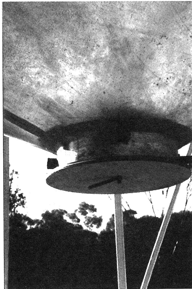
Fig. 9. Sealing plate for a butterfly grain control.
