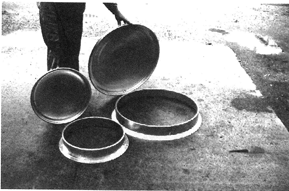
Fig. 7. Spun lids with rolled welded band.
