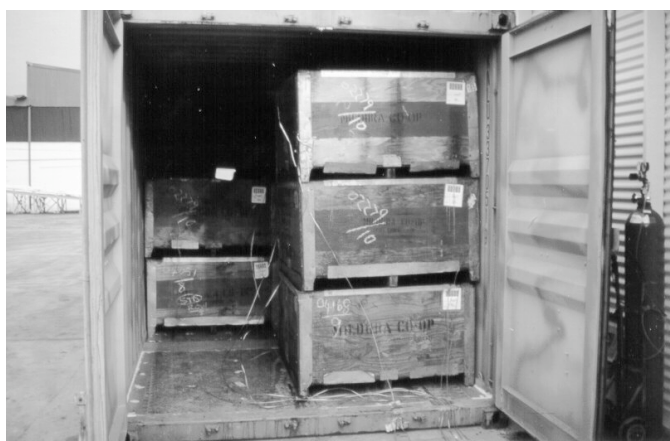
Figure 1. Shipping container with 0.5t bins and sample lines prior to addition of ethyl formate
