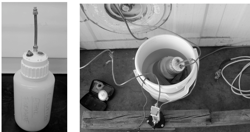
Figure 4. a (left): Experimental ethyl formate dosing vessel, b (right): ethyl formate dosing vessel attached to CO 2 gas flow via copper lines and kept warm in water bath during gas addition.
