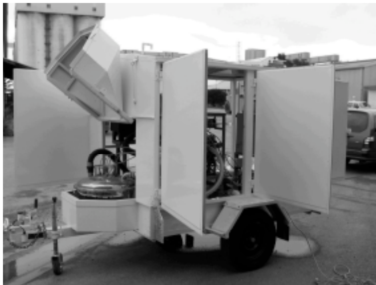
Figure 3. Charcoal scrubber designed to safely remove residual production of phosphine during an unscheduled shutdown of the generator.
