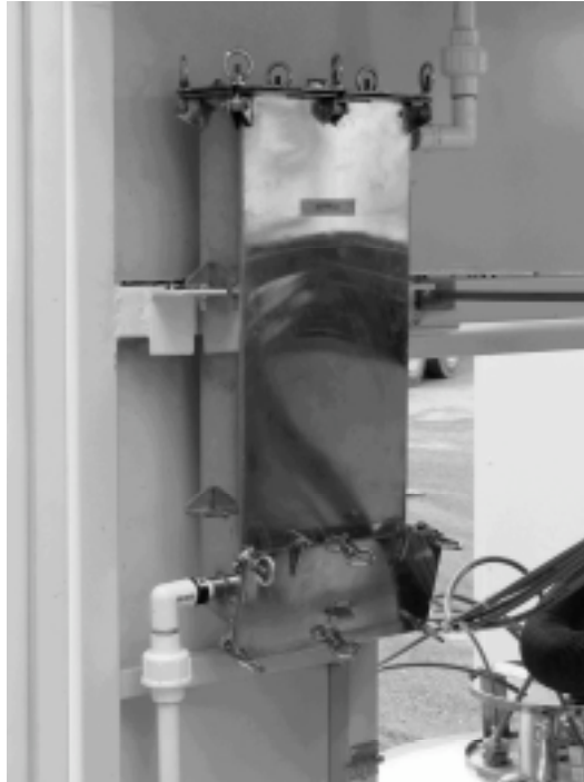
Figure 3. Charcoal scrubber designed to safely remove residual production of phosphine during an unscheduled shutdown of the generator.
