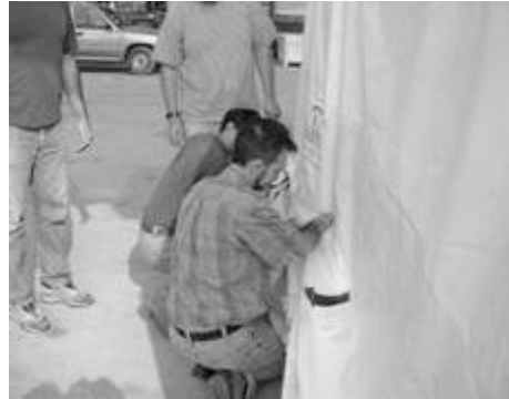
Figure 8 – Joining the top and the bottom sections of the V-HF Cocoon using the zipper.
