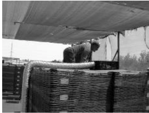
Figure 6 – Locating the heat source inside the plenum on top of stack and connecting it to circulation duct.
