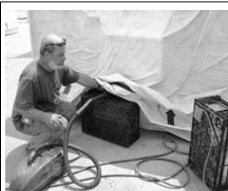
Figure 9 – Creating a low pressure of -200 Pa in the V-HF Cocoon using a vacuum cleaner.
