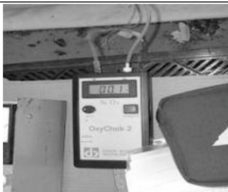
Figure 10 – Recording the generated low oxygen (0.1%) atmosphere in the V-HF Cocoon.
