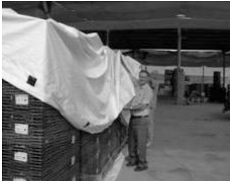
Figure 7 – Closing the V-HF Cocoon with the top section cover.
