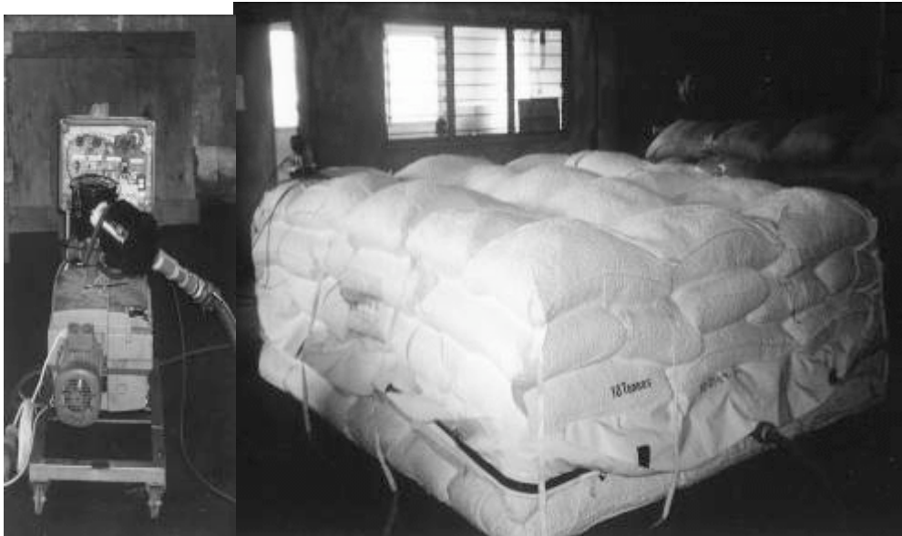
Figure 15. GrainPro Cocoon™ containing cocoa beans used as vacuum cube during the trials in Ivory Coast. The rotary oil-lubricated vacuum pump is shown on the left of the picture.
