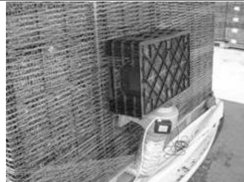
Figure 4 – Placing the circulation fan below empty box to form plenum.
