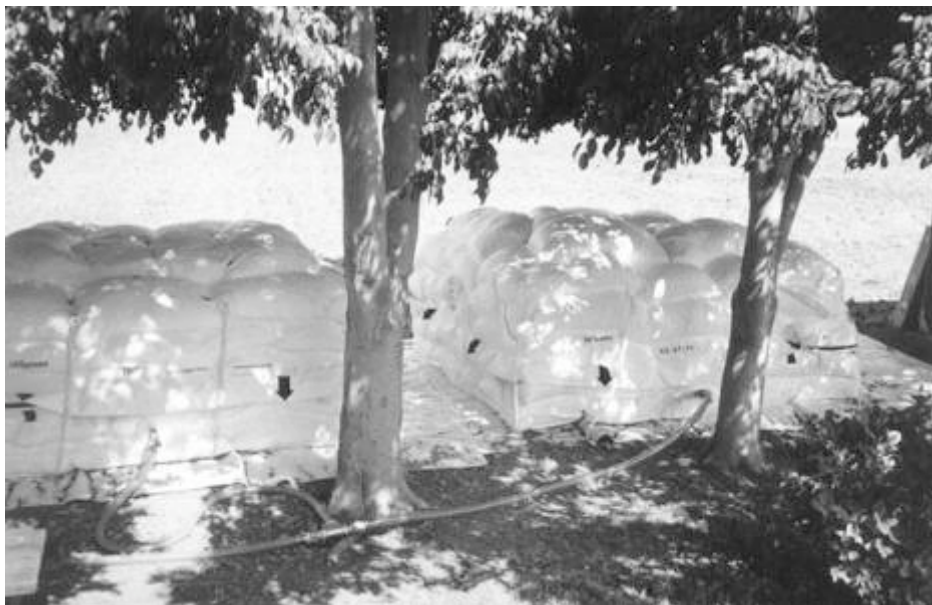
Figure 14. Two Volcani Cubes™ under a pressure of 50 mm Hg (3 days exposures on the right and 7 day exposures on the left) connected together to the pump at the trial site in Israel.
