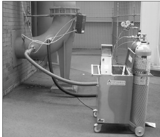
Figure 1. The HORN DILUPHOS SYSTEM® setup for fumigation.
