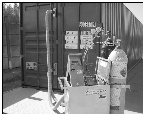
Figure 11. Container being fumigated with the HDS together with the JP- System.
