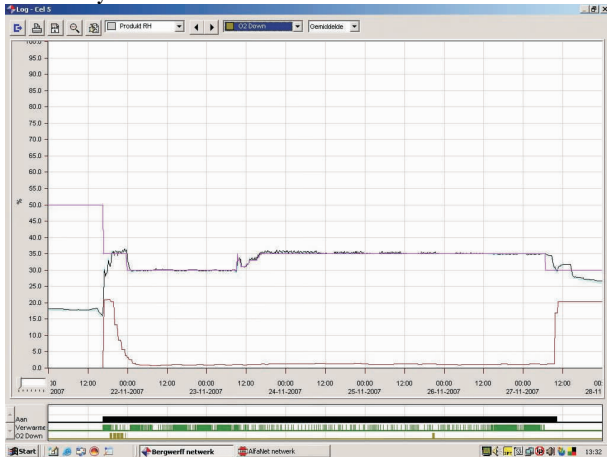
Fig. 7 Treatment graphic (black line = inlet temperature, blue line = room temperature, red line = O 2 concentration, pink line = set point temperature)
