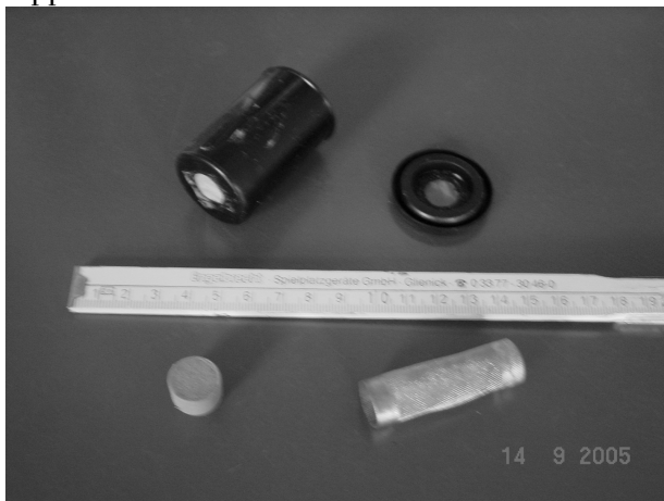
Fig. 2 Film boxes with stainless steel gauze
