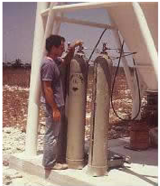
Fig. 4 For small-scale applications of up to 50 tonnes capacity containers, pressurized cylinders are sufficient.
