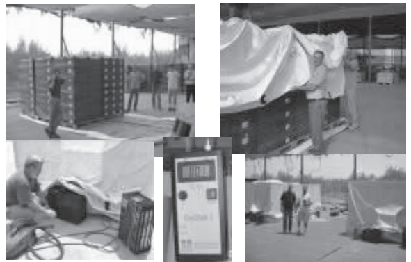
Fig. 5 Bio-generated modified atmosphere for the control of narcissus fly utilizing the bulb respiration alone in specially designed flexible treatment chambers.
