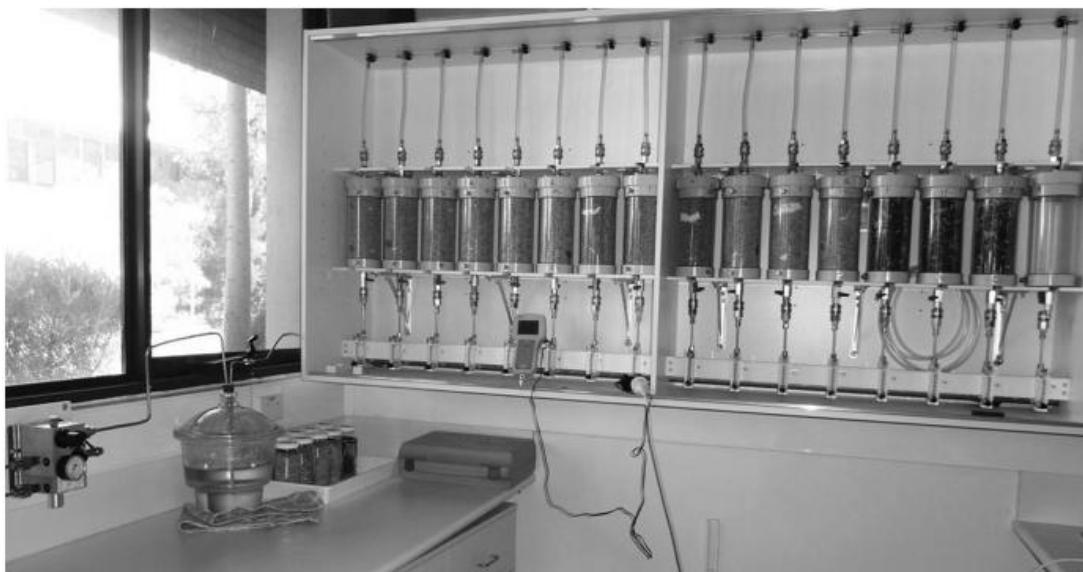
Fig 1- A gas purging flow system was used to treat the insects with constant concentrations of nitrogen and oxygen and maintained low carbon dioxide concentrations during the period of treatment. All 15 cylinders were filled with a known amount (1.8-2 kg) of grain (wheat, barley, oats, lupin and canola).
