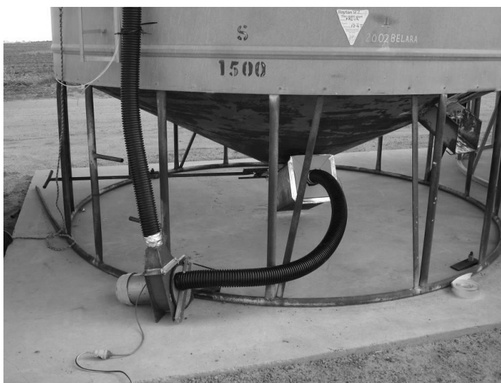
Fig. 1- Fan connected to base and headspace of silo by a 90mm i.d. flexible pipe.
