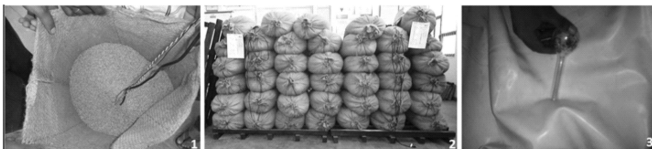
Fig. 6. Sensor rod installation in a gunny bag 1 , Gunny bags piles on wooden crates 2 and manual insect infestation 3 of the hermetic bag.
