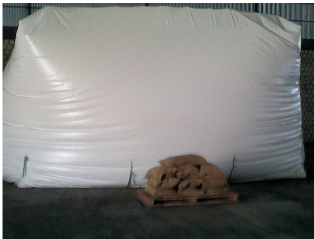
Fig. 3. Ballooning effect at the end of purging CO 2 on 300 tonnes of basmati milled rice stored in G-HF Cocoon in KFM warehouse in Kuwait
