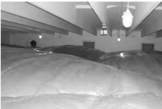
Fig. 3. The grain bulk covered by air tight liner for maintaining N_2 atmosphere.
