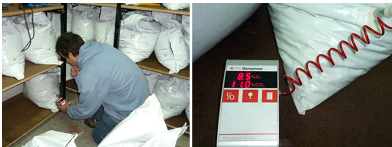
Fig. 2. Measuring O 2 and CO 2 concentrations
