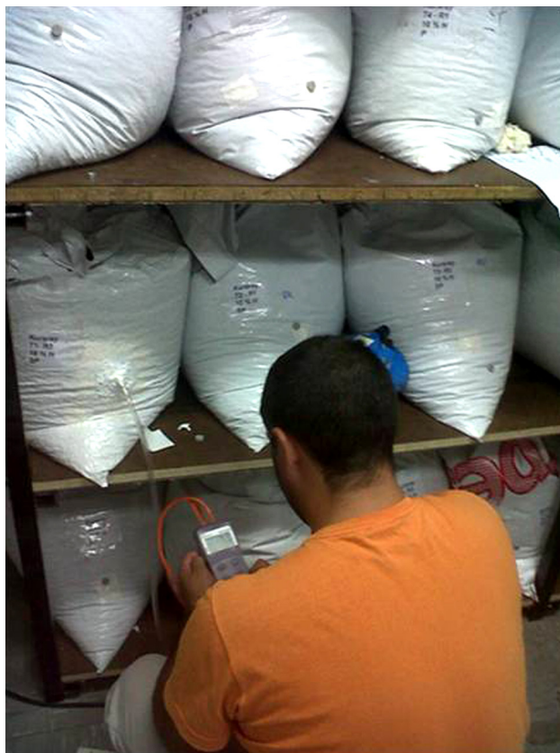
Fig. 1. Performing a pressure decay test in the experimental bags
