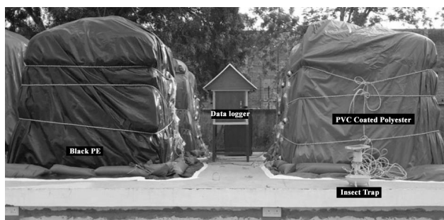
Fig. 1. Effect of PVC coated polyester cover on paddy storage
