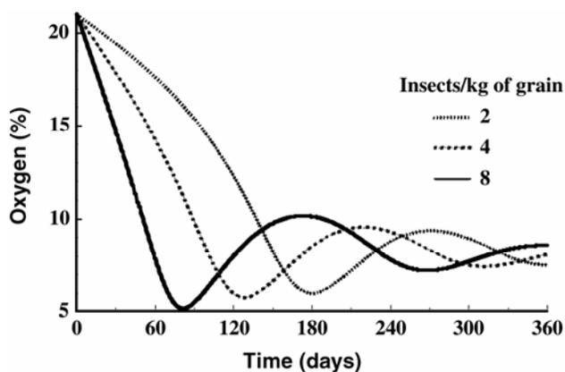
Fig. 13. Calculated oxygen concentrations in a 10-m<sup>3</sup> grain mass containing different infestation levels of insects and having an oxygen intake of 157  $\mu$ L per insect per day, using a sealed liner with an oxygen ingress rate of 0.24% per day. (Redrawn, and used with permission, from Navarro et al, 1994)
