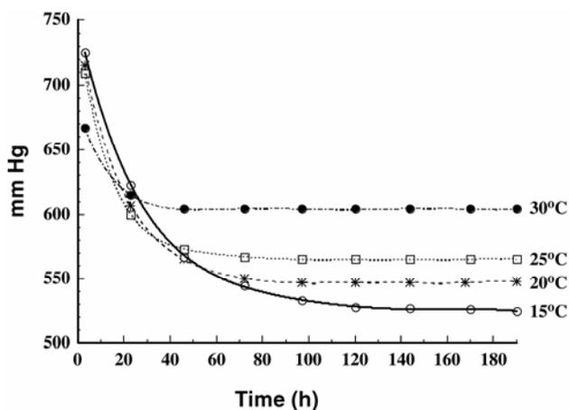
Fig. 11. Pressure decay due to sorption of CO<sub>2</sub> in gastight containers filled to 93% capacity with wheat at four temperatures, with an initial CO<sub>2</sub> concentration of 99.8% and an initial pressure of 768 mm of Hg. (Redrawn, and used with permission, from Navarro, 1997b)
