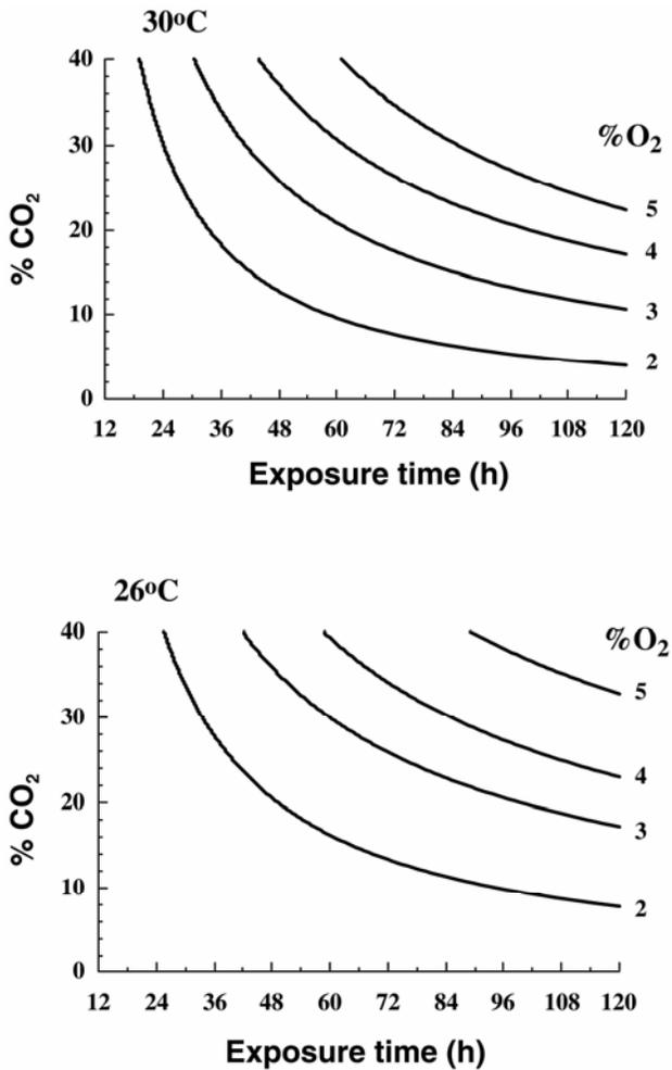
Fig. 4. Calculated exposure times and carbon dioxide levels to produce 95% mortality for *Tribolium castaneum* adults at four oxygen concentrations and two temperatures at 57% RH. (Redrawn, and used with permission, from Calderon and Navarro, 1979)
