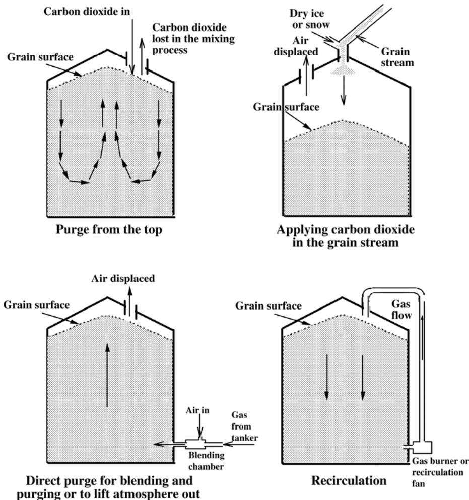
Fig. 12. Four methods of applying a modified atmosphere.
