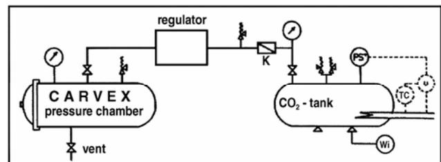
Fig. 14. Pressure chamber of about 3 m<sup>3</sup> designed to hold CO<sub>2</sub> at 20 and 37 bar, liquid CO<sub>2</sub> supply tank, and regulator unit. (Reprinted, with permission, from Gerard et al (1990))
