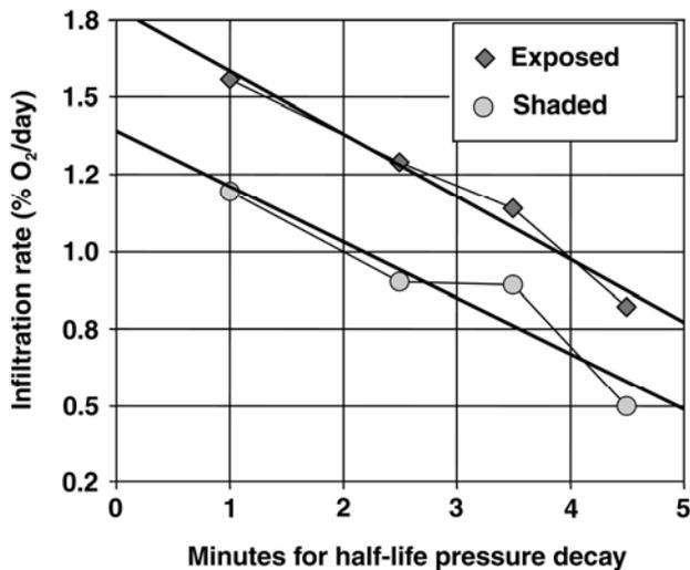
Fig. 17. Infiltration rate of oxygen into a nitrogen-treated empty structure of 7.5-m<sup>3</sup> capacity in relation to half-life pressure-decay time. The suggested maximum infiltration rate for modified atmospheres is an increase of 0.5% O<sub>2</sub> per day. (Data from Navarro and Zettler, 2001)
